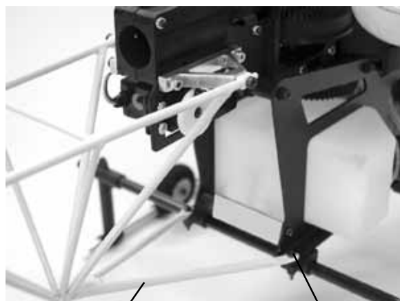
Tail Truss Assembly [CN1074-10] M3x12 Self Tapping Screws x 4
